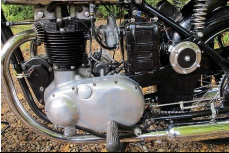
1952 A7 Star Twin. Note the sensible upgrade to an Amal Concentric carburettor. Not sure about the horn either, but who cares? Lovely bike
